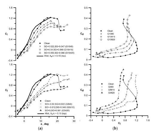
**Figure 7.** Effect of slat gap and angle on the (**a**) measured lift coefficient and (**b**) profile drag coefficient with side plates installed.
