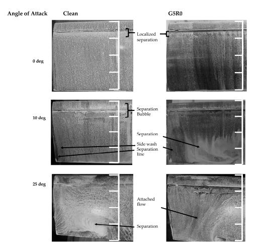
**Figure 4.** Effect of angle of attack and slat deployment (G5R0 geometry) on surface skin friction patterns. Flow is from top to bottom. Ruler divisions are one-quarter chord.
