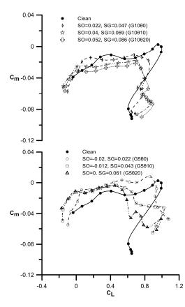
Figure 6. Effect of slat gap and angle on pitching moment coefficient.
