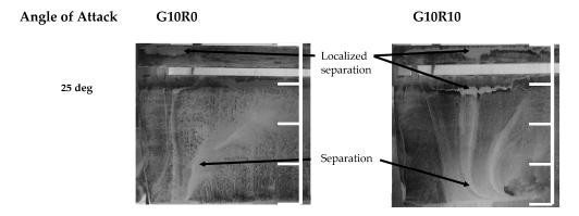
**Figure 5.** Effect of angle of attack and slat deployment (G10R0 and G10R10 geometry) on surface skin friction patterns. Flow is from top to bottom.
