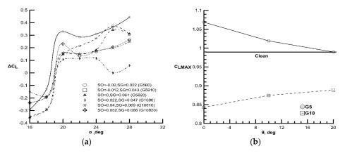
**Figure 3.** Effect of slat gap and angle on (**a**) the lift increment relative to the clean wing and (**b**) the maximum lift coefficient.
