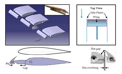
**Figure 1.** Rendering showing wind tunnel model construction, model sting installation (inset), side plate installation, airfoil profile and slat variable definitions.
