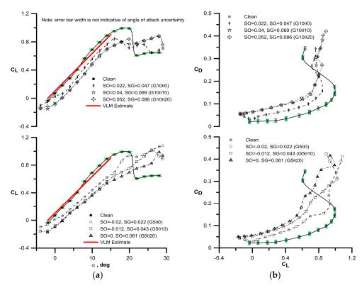
**Figure 2.** Effect of slat gap and angle on the (**a**) measured lift coefficient and (**b**) drag coefficient, error bars are shown in green.
