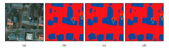
**Figure 8.** Results of the building extraction in the urban district of the Potsdam dataset with and without edge enhancing preprocessing. (**a**) The original imagery of this urban district. (**b**) The ground truth of this region. (**c**) The prediction results using the Res-U-Net without enhanced preprocessing. (**d**) The prediction results with enhanced preprocessing.
