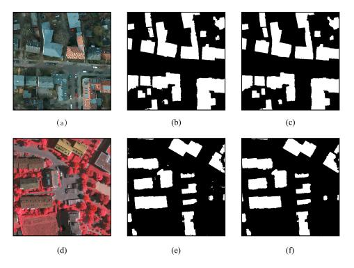
**Figure 6.** Results of the guided filter. (**a**) represent the original imageries in the Potsdam and Vaihingen datasets, respectively. (**b**) represent the corresponding prediction from deep learning. (**c**) represent the results of guided filter. (**d**–**f**) are the original imageries, prediction from deep learning and the results of guided filter in Vaihingen, respectively.
