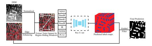
Figure 1. The framework of the pixel classification using deep learning and a guided filter.
