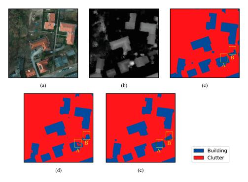
**Figure 9.** The results of the building extraction in the urban district of the Potsdam dataset with and without the DSM as a channel of the input. (a) The original imagery of the urban district. (b) The DSM of this district. (c) The ground of this region. (d) The prediction results using the Res-U-Net without the DSM as a channel of input. (e) The prediction results corresponding to the input with the DSM.
