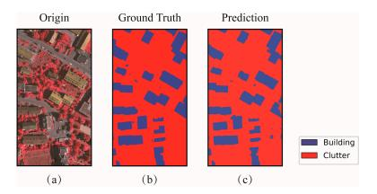
**Figure 5.** Results of the buildings extraction of the Vaihingen dataset using deep learning, the imagery (**a**) as well as the corresponding ground truth (**b**) and the prediction (**c**).
