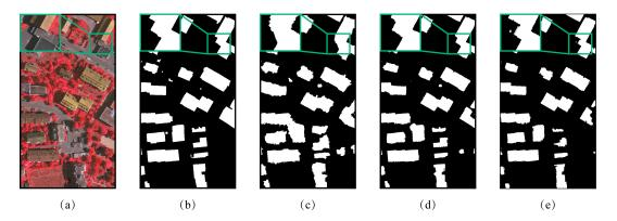
**Figure 11.** The results of the guided filter. (a) The imagery of the urban district. (b) The ground truth corresponding with the imagery. (c) The optimization result with a guided filter with a threshold t = 40. (d) The optimization result with a guided filter with a threshold of t = 90. (e) The optimization result with a guided filter with a threshold of t = 165.
