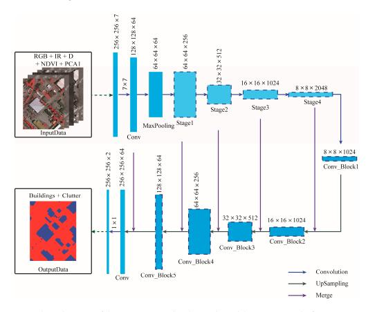
**Figure 2.** The architecture of the Res-U-Net used in this work. Each box represents the feature map and the x-y-size of the map is provided at the lower right edge of the box. The arrows denote the different operations which are explained at the lower right of the figure.
