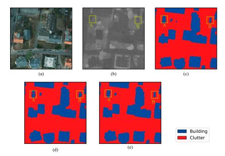
**Figure 10.** The results of the building extraction in the urban district of the Potsdam dataset with and without the NDVI as a channel of the input. (**a**) The original imagery of the urban district. (**b**) The NDVI of this district. (**c**) The ground of this region. (**d**) The prediction results using the Res-U-Net without the NDVI as a channel of input. (**e**) The prediction results corresponding to the input with the NDVI.
