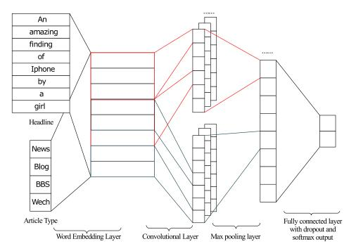
Figure 2. The structure of the clickbait convolutional neural network.
