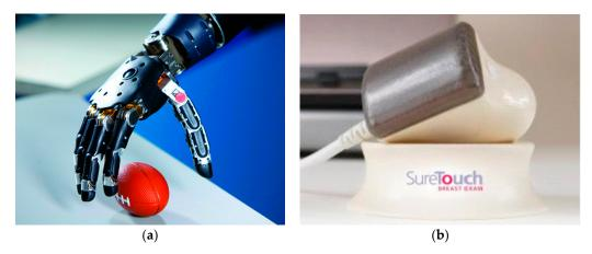
**Figure 2.** Two examples of tactile sensing systems for biomedical engineering: (**a**) the modular prosthetic limb; and (**b**) the SureTouch sensor for breast exam [120,121] (Reprinted with permission. Copyright 2015 IEEE).
