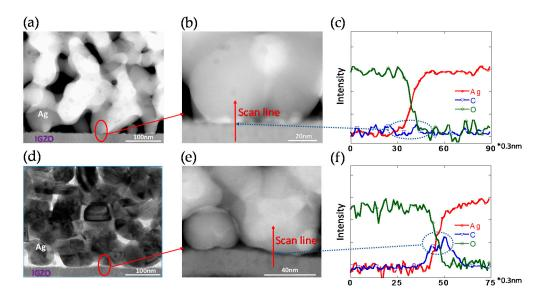
**Figure 5.** Comparision of Ag/a-IGZO interfaces for silver salt and nanoparticles inks. (a) TEM image of the silver/a-IGZO structure for silver salt ink; (b,c) Respectively show the amplified area and the EELS measurement of Ag, C, and O along marked scan line; (**d**–**f**) TEM images and the ELLS measurement for the nanoparticles ink.
