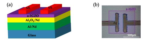
**Figure 1.** (**a**) Schematic of a-IGZO TFT with inkjet printing Ag S/D electrodes; (**b**) Optical microscope image of device finally fabricated.
