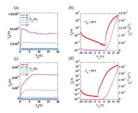
**Figure 4.** (**a**) Output and (**b**) transfer characteristics of the device with silver nanoparticle ink; (**c**) Output and (**d**) transfer characteristics of the device with silver salt ink.
