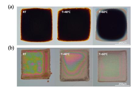
**Figure 2.** Inkjet printed with (**a**) silver nanoparticles ink film and (**b**) silver salt ink film on a-IGZO/Al<sub>2</sub>O<sub>3</sub> with substrate temperatures of RT, 40 °C and 60 °C, respectively.
