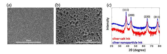
**Figure 3.** SEM images of the inkjet printed silver electrodes of TFTs by using (**a**) silver nanoparticles ink and (**b**) silver salt ink, respectively; (**c**) XRD patterns of the silver films after thermal treatment.
