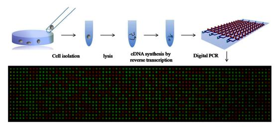
**Figure 9.** Self-priming compartmentalization (SPC) digital PCR chip for single-cell gene expression. Reprinted from [191], with the permission of AIP Publishing.
