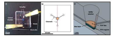
**Figure 5.** (a) Microfluidic device used to perform integrated DNA purification and amplification experiments; (b) schematic top view of the channels and central chamber; (c) schematic cross section view of FTA<sup>®</sup> paper discs placed on top of a layer of wax-encapsulated PCR. Reproduced with permission from [80].
