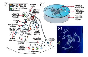
**Figure 13.** Lab on disc: (**a**) Schematic of lab on a disc with DNA extraction and purification using beads packed inside a microchannel, LAMP reservoir for multiplexed amplification; (**b**) assembly of the disc with patterned PMMA layer; (**c**) fully assembled lab-on-a-disc. Reproduced from [232] with permission of The Royal Society of Chemistry.
