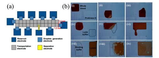
**Figure 14.** Digital microfluidic chip for DNA extraction. (a) Schematic of DMF chip; (b) Extraction process: (**i**–**iii**) degradation of nucleases using proteinase K; (**iv**–**vi**) lysis buffer was added to the droplet; (**vii**,**viii**) binding of DNA with beads; (**ix**) the mixture was mixed in a loop motion to obtain a uniform droplet color. Reproduced from [237] with permission of Springer.
