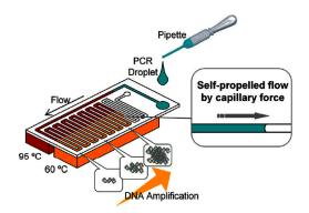
**Figure 8.** Schematics of self-propelled CF-PCR microfluidic device. The PCR solution is dropped and automatically transported by capillary forces. Reproduced with permission from [123]. Copyright (2015), with permission from Elsevier.
