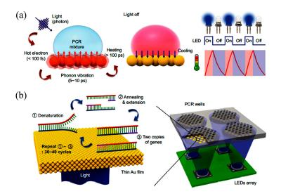
**Figure 7.** Ultrafast photonic PCR (**a**) Schematic of the plasmonic photothermal induced heating of the PCR mixture; (**b**) schematics of the ultrafast photonic PCR using a thin gold (Au) film cycling with LED arrays. Reprinted from [108] with permission of Nature Publishing Group, Copyright 2015.
