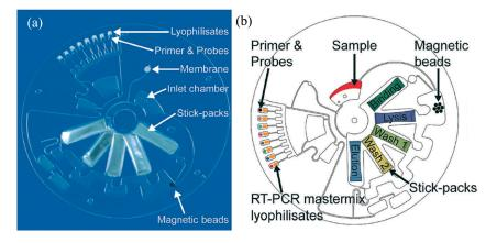
**Figure 16.** (a) Photograph of the LabDisk for respiratory pathogens with complete reagent prestorage; (b) schematic of device with sample supplied into the LabDisk—automated to pump the sample into the lysis chamber by centrifugation and therein with prestored magnetic beads. Finally, reverse transcription and PCR with real-time fluorescent readout are performed. Reproduced from [250] with permission of The Royal Society of Chemistry.
