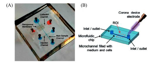
**Figure 4.** Electrical lysis: (**A**) electrical lysis using nanoporous membrane; Reproduced with permission from [60]. (**B**) Schematic of the experimental setup using corona discharge. Reproduced from [61] with permission of The Royal Society of Chemistry.
