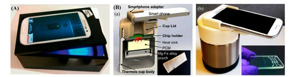
**Figure 10.** (**A**) NAIL mobile imaging unit consisting of a dark box with an excitation and emission filter, and mobile phone. Reproduced from [149] with permission of The Royal Society of Chemistry. (**B**,**a**) Exploded view of smart cup. Inset is a snapshot of the Mg–Fe alloy pouch used as a heating source. (**b**) A photograph of a fully assembled smart cup. Inset is a snapshot of an integrated microfluidic chip. Reprinted from [209]. Copyright (2016), with permission from Elsevier.
