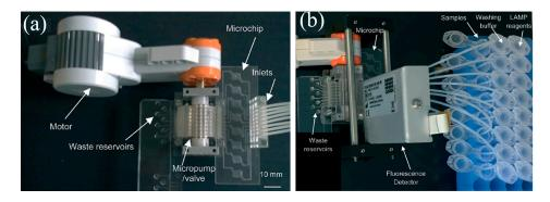
**Figure 15.** (a) Integration MainSTREAM micropump with microchip; (b) an eight-chamber microfluidic chip was connected with eight-channel peristaltic micropump to load the sample and reagents, integrated with a fluorescence detector. Reproduced from [246] with permission of The Royal Society of Chemistry.
