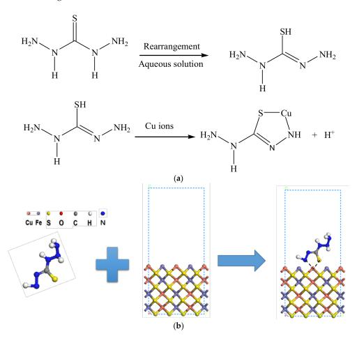
**Figure 11.** (a) Rearrangement of functional group NH<sub>2</sub>–NH–C(–SH)=N–NH<sub>2</sub> and formation of complexes on chalcopyrite surface; (b) proposed chemisorption model of TCH on chalcopyrite surfaces.
