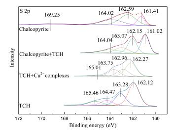
Figure 7. S 2p spectra of TCH, TCH–Cu<sup>2+</sup>, and chalcopyrite before and after treatment.
