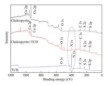
Figure 6. XPS spectra of TCH and chalcopyrite with and without treatment.
