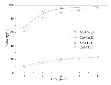
Figure 3. Flotation recovery of Cu and Mo at different flotation time with different depressants.
