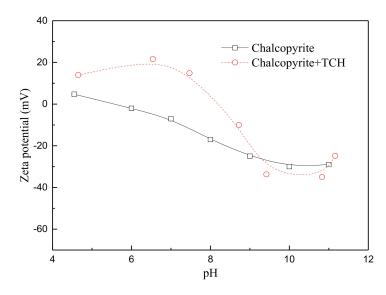
**Figure 4.** Zeta potential measurements of pure chalcopyrite as a function of pH in presence and absence of TCH ( $2 \times 10^{-4}$  M/L).
