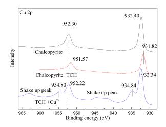
Figure 9. Spectra of TCH+Cu<sup>2+</sup> complexes, chalcopyrite before and after treatment.
