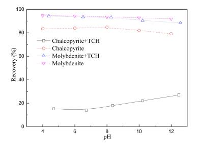
**Figure 2.** Influence of pH on floatability of chalcopyrite and molybdenite with or without thiocarbonohydrazide ( $4 \times 10^{-4} \text{ mol/L}$ ), MIBC (80 mg/L) and Kerosene (200 mg/L).
