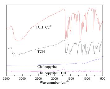
Figure 5. FTIR spectra of TCH, TCH–Cu<sup>2+</sup> complexes and chalcopyrite treated and untreated with TCH.
