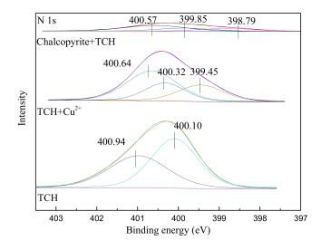
Figure 8. N 1s spectra of TCH, TCH–Cu<sup>2+</sup> and chalcopyrite after treatment.
