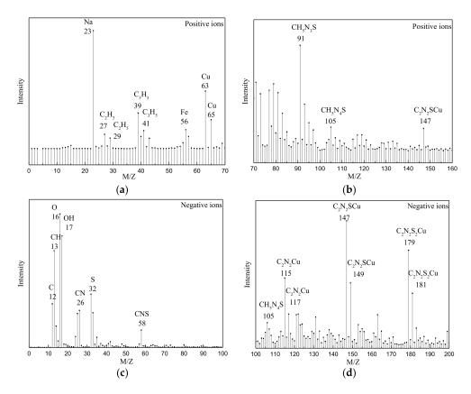
**Figure 10.** ToF-SIMS spectra of chalcopyrite surface after adsorption of thiocarbonohydrazide, (**a**,**b**) negative-ions; and (**c**,**d**) positive-ions spectra.
