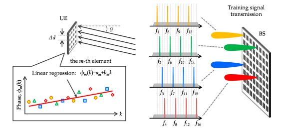
Figure 3. Proposed high efficient channel state information (CSI) estimation.
