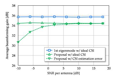
Figure 11. Average beamforming gain versus signal-to-noise power ratio (SNR).
