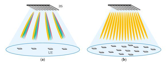
**Figure 1.** System model: (a) Multistream transmission per user equipment (UE): Nu = 4 and Ns = 4; and (b) 1st eigenmode transmission per UE: Nu = 16 and Ns = 1.
