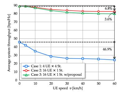
Figure 9. Average system throughput versus UE speed.
