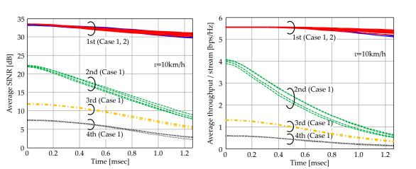
**Figure 4.** Time variant characteristics within the CSI estimation period. Case 1: Nu = 4, Ns = 4; Case 2: Nu = 16, Ns = 1. (a) Average SINR per stream versus elapsed time. (b) Average throughput per stream versus elapsed time.
