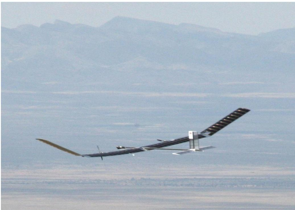
HALE UAS platforms are primarily valuable for strategic observation of large-scale (global/continental) phenomena where other platforms do not have the flight characteristics to support extensive mission operations. Platforms like the Global Hawk and the Zephyr (and other, similar platforms currently in development) will see increased use in atmospheric studies, and there are indications that HALE platforms in the next few years could provide near-continuous coverage of the
