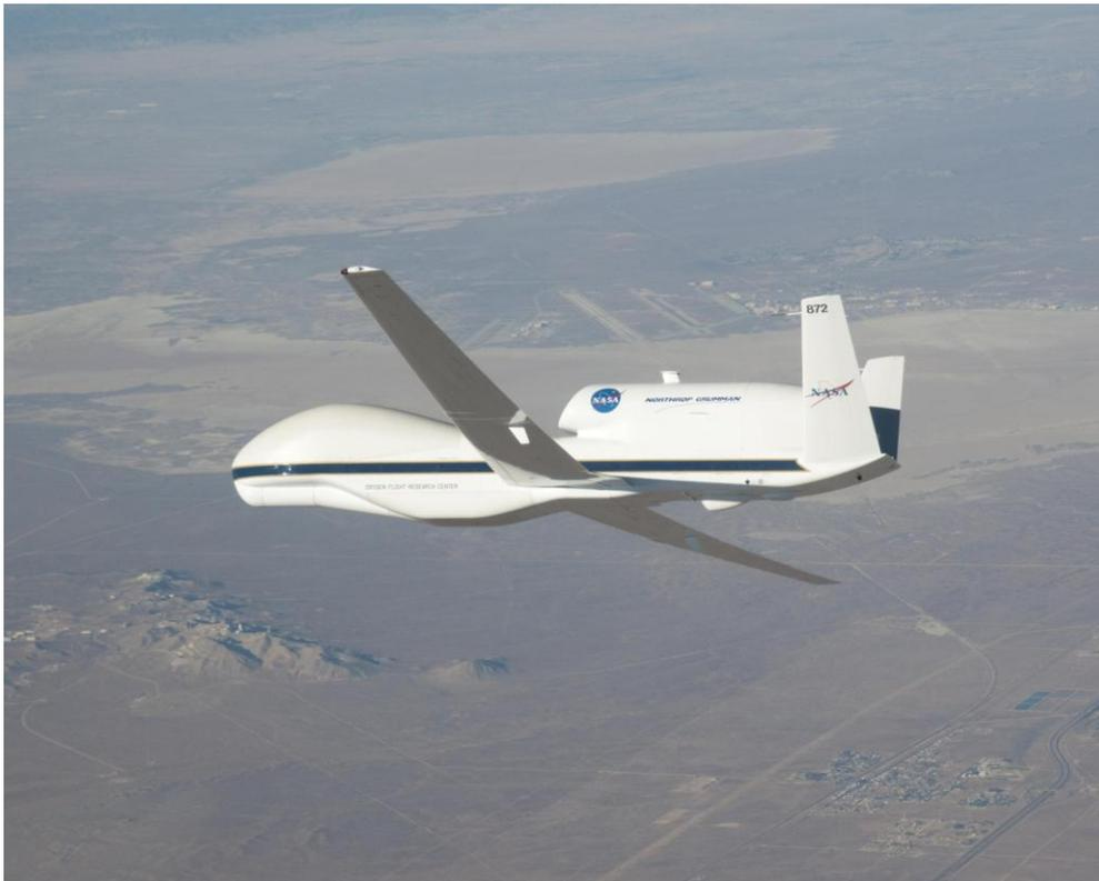
The 2010 Global Hawk Pacific Mission (GloPac) campaign was the first NASA Earth Science campaign to be conducted on the aircraft. Ten instruments were installed in the HALE UAS to support measurements of trace gases, aerosols and dynamics of the upper troposphere and lower stratosphere. The instrumentation also supported validation efforts of the instruments aboard the NASA Aura and CALIPSO earth-monitoring satellite.
