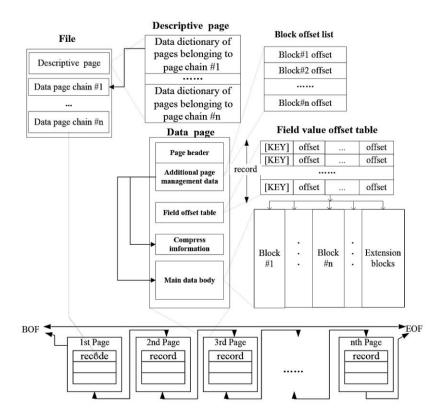
Figure 3. Physical structure of the China Navigation Data Format (CNDF).
