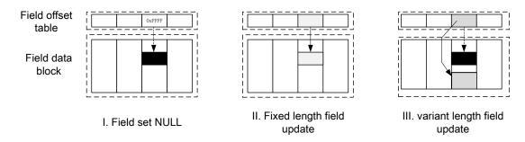
Figure 5. Field update mechanism in real-time data update method.
