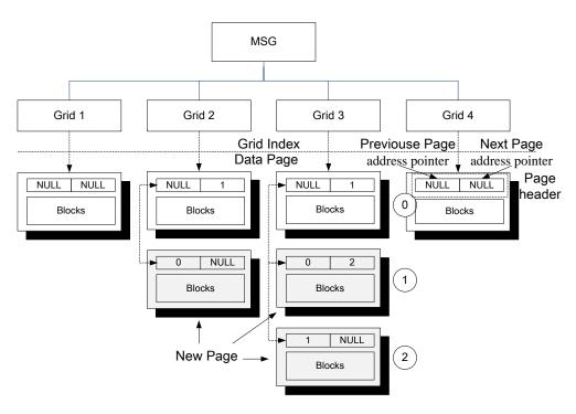
Figure 6. Incremental update mechanism in incremental data update method.
