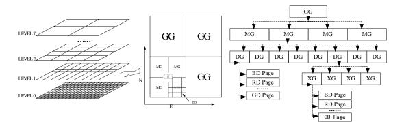
Figure 1. Illustration of the Multi-Scale Grid index.
