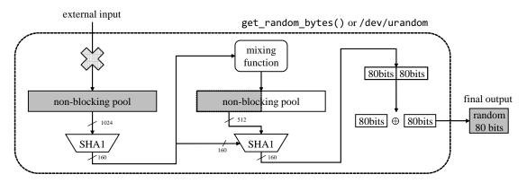
**Figure 2.** *Extract unit*: Extracting random numbers using get\_random\_bytes() or /dev/urandom without the entropy transfer.
