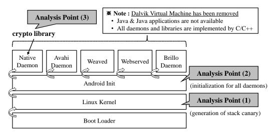
Figure 3. Structure of Brillo and three analysis points.
