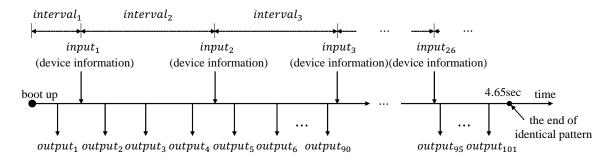
Figure 8. Timeline for identical pattern at boot time in Brillo.
