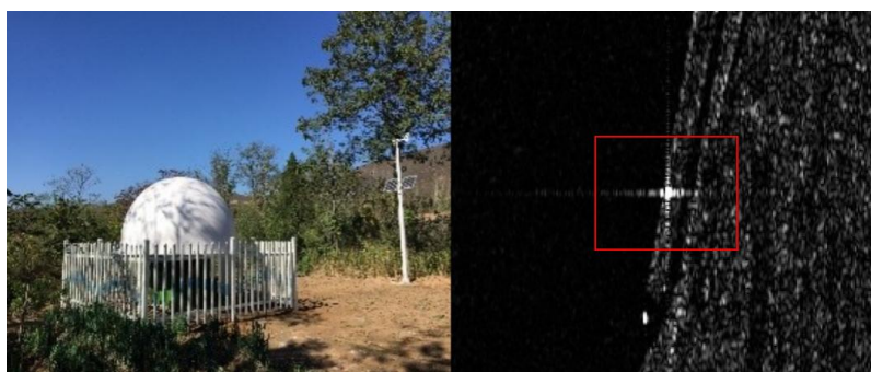
Figure 5. Appearance of the corner reflector (left) and its image performance (right).
