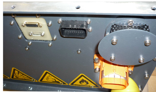
Figure 2: Front of the housing with the IP compatible HV-plug and the vent at the right hand side
