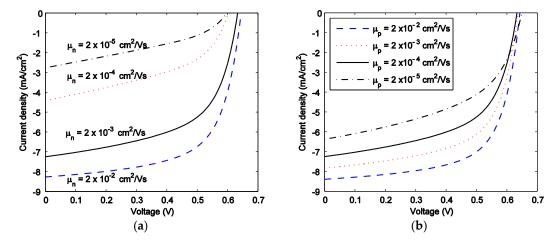
Figure 9. Theoretical current-voltage characteristics of P3HT:PCBM solar cells for (a) varying electron mobility with  $\mu_p = 2 \times 10^{-4} \text{ cm}^2/\text{Vs}$  and (b) varying hole mobility with  $\mu_n = 2 \times 10^{-3} \text{ cm}^2/\text{Vs}$ . Carrier lifetimes are:  $\tau_n = \tau_p = 20 \ \mu \text{s}$ .
