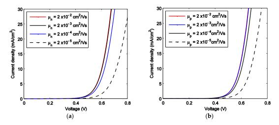
**Figure 4.** Theoretical dark current-voltage characteristics of P3HT:PC<sub>61</sub>BM solar cells for (a) varying  $\mu_v$  with  $\mu_v = 2 \times 10^{-4}$  cm<sup>2</sup>/Vs and (b) varying  $\mu_v$  with  $\mu_v = 2 \times 10^{-3}$  cm<sup>2</sup>/Vs.
