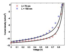
**Figure 6.** Current-voltage characteristics of PCDTBT solar cells for different active layer thicknesses. The symbols and solid lines represent experimental data and model fit to the experimental data, respectively.
