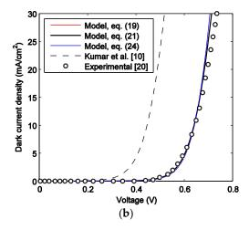
**Figure 2.** Dark current-voltage characteristics of P3HT:PCBM solar cells. (**a**) The experimental data are extracted from Reference [19]; and (**b**) The experimental data are extracted from Reference [20].
