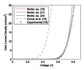
**Figure 3.** Dark current-voltage characteristics of a PTB7:PC<sub>71</sub>BM solar cell.
