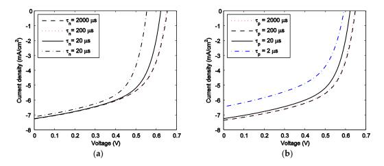
**Figure 10.** Theoretical current-voltage characteristics of P3HT:PCBM solar cells for (**a**) varying electron lifetimes with  $\tau_p = 20~\mu s$  and (**b**) varying hole lifetime with  $\tau_n = 20~\mu s$ . Carrier mobilities are:  $\mu_p = 2 \times 10^{-4}~\text{cm}^2/\text{Vs}$  and  $\mu_n = 2 \times 10^{-3}~\text{cm}^2/\text{Vs}$ .
