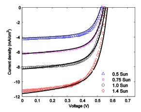
**Figure 5.** Current-voltage characteristics of a P3HT:PCBM solar cell at different sun intensities. The symbols represent experimental data and solid lines represent the model fit to the experimental data.
