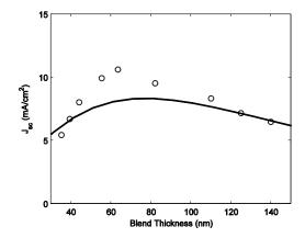
**Figure 7.** Short circuit current density ( $J_{sc}$ ) *versus* active layer thickness (L). Symbols: experimental data and solid line: model fit to the experimental results.
