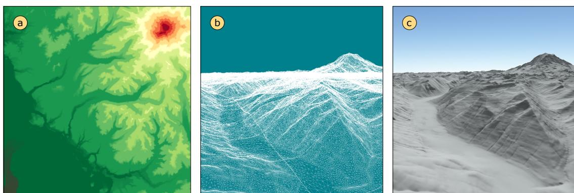
**Figure 1.** Visualizing 3D terrain. The terrain model is typically based on height-field data (a) from which triangular networks are generated (b) before the final model is rendered (c).
