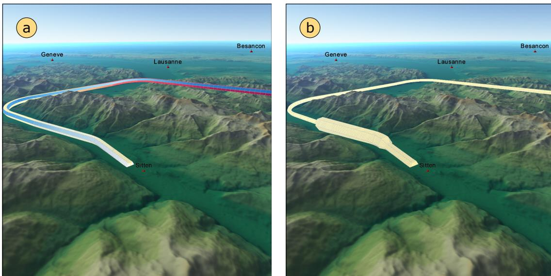
**Figure 12.** Communicating further details of the trajectory. The image on the left (a) depicts two parameters encoded into color: wind speed (yellow to red) and the amount of cross wind (light blue to dark blue). The image on the right (b) shows outliers in fuel consumption along the path by the width of the trajectory (greater width means larger fuel consumption).
