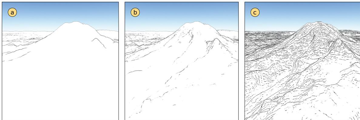
**Figure 4.** Enhanced edges using line drawing: (a) silhouettes are emphasized; (b) additional contours along ridges are drawn and (c) additional suggestive contours are drawn.
