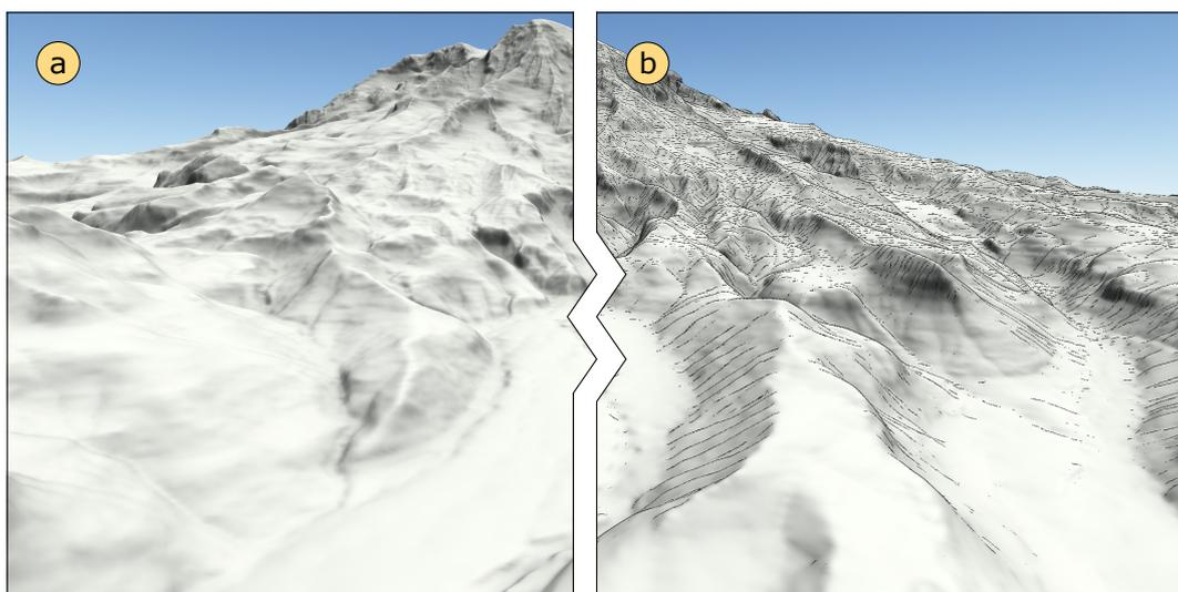
**Figure 5.** Shaded surfaces (a) can be extended with enhanced edges (b) to emphasize contour-based features of the terrain.
