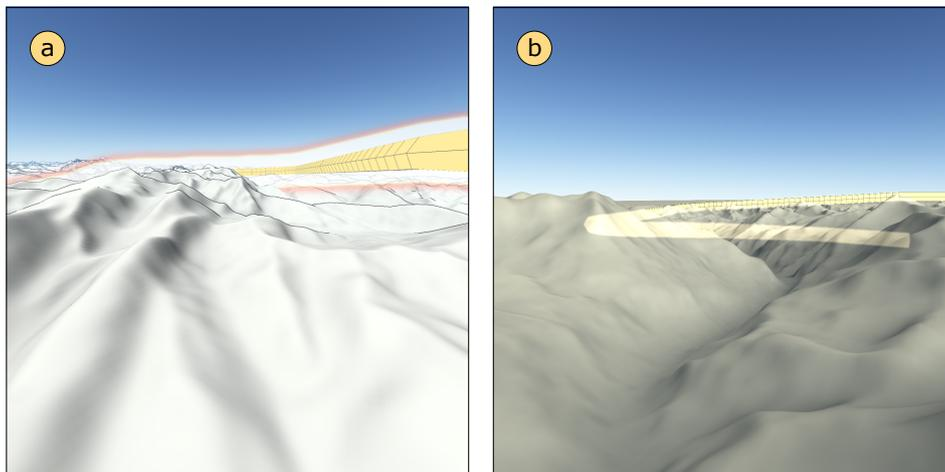
**Figure 11.** Improving communication of the position and path of the trajectory. (a) depicts a halo around the trajectory to increase its prominence; in (b), the geometry of the trajectory shines through the terrain if it is occluded.
