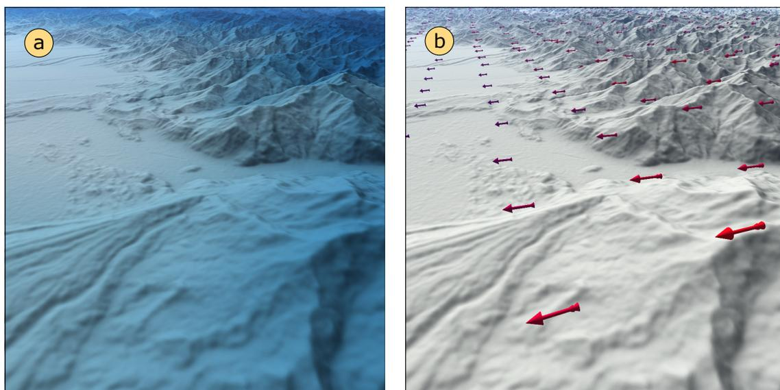
**Figure 7.** Visualizing data together with terrain. (a) shows relative humidity encoded into the color of the surface (light blue means low humidity, dark blue means high humidity); (b) shows wind glyphs, encoding wind direction and strength. The direction is given by the arrow head and the strength is encoded by the length of the arrow and a continuous color scale, ranging from blue (light wind) to red (high wind).
