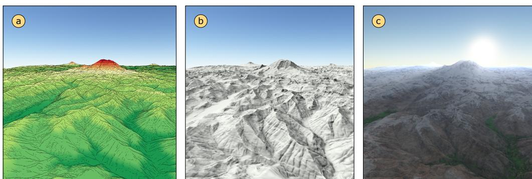
**Figure 16.** Visualizing terrain using different render methods and parameters: In (a), edge enhancement combined with elevation-coloring is used; in (b), a global illumination model is applied, and, in (c), volumetric lighting is added.
