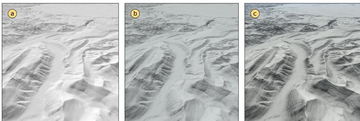
**Figure 3.** Conveying fine 3D structures of the terrain surface using different illumination models: (a) local illumination; (b) local illumination combined with ambient occlusion; and (c) global illumination.
