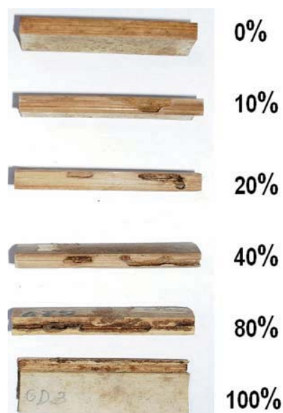
Figure 2. Visual rating of termite attack on bamboo test blocks.
