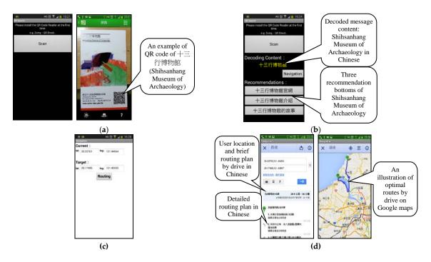
**Figure 3.** Dr. What-Info system outcomes. (**a**) Picture of reading the QR/bar code; (**b**) results of recognition and appropriate recommendations; (**c**) selection and presentation of local GPS; (**d**) and planning and presentation of target path.
