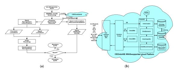
**Figure 2.** Prototype system of Dr. What-Info. (**a**) Operation of the fore-end system; and (**b**) architecture of back-end system.
