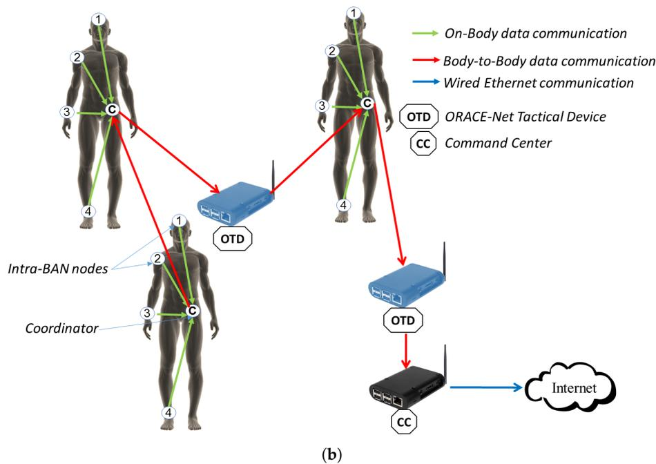
**Figure 2.** (a) CROW<sup>2</sup> system layer-based architecture. BT: Bluetooth, ZB: ZigBee, WF: WiFi, WB: WBAN. For the CROW<sup>2</sup> system, we considered Bluetooth between sensors and the coordinator and WiFi IEEE802.11n between WBANs and the Command Center node (CC node). (b) Multi-hop aspect in CROW<sup>2</sup>; Data are routed from/through mobile/tactical nodes towards the Internet. MQTT, Message Queuing Telemetry Transport.
