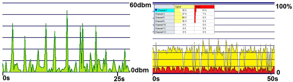
**Figure 11.** (a) Interference score (in dBm) recorded over 25 s on the channel at 2.412 GHz (AirMagnet WiFi Analyzer Limited Edition). (b) Screen-shot of signal and noise (as a percentage) recorded over 50 s (AirMagnet WiFi Analyzer Limited Edition).
