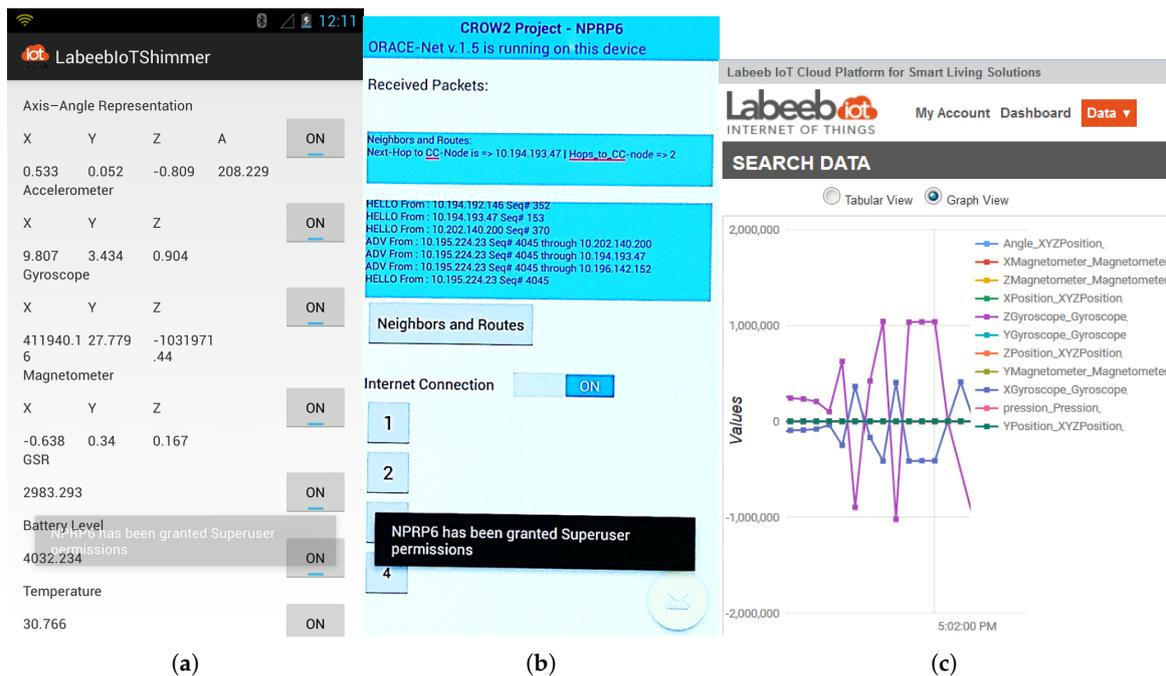
**Figure 4.** (a) A screen-shot from the Labeeb-IoT Shimmer sensing mobile app, which collects data from Shimmer [31] sensors and pushes them to the Internet of Things platform (Labeeb-IoT). (b) Testbed: a photo of the ORACE-Net mobile devices displaying the real-time events (received "Hello" and Advertisement ("ADV") packets) and the current route. (c) The Labeeb-IoT [32] interface shows the variation of the sensed data from the Shimmer sensor connected to the mobile node.
