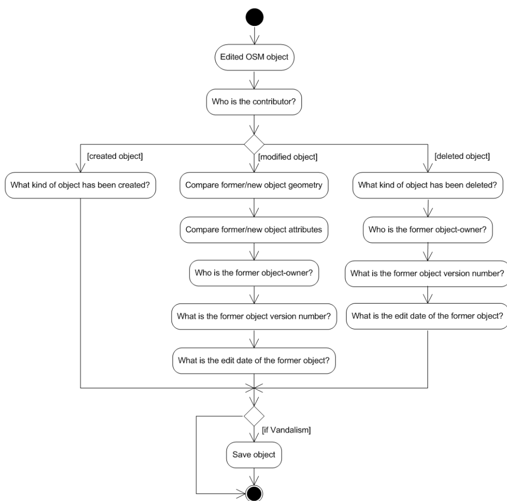
Figure 5. UML activity diagram to detect the types of vandalism of an OSM edit sequence diagram of the vandalism detection tool ( OSMPatrol ).
