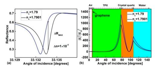
**Figure 6.** (a) Shift of Fano lineshape for the structure with  $d_1 = 7 \ \mu m$ ,  $d_2 = 70 \ \mu m$ ,  $E_F = 0.35 \ eV$ ; (b) Schematic diagram of the electric field distributions for the proposed Fano resonance sensor at  $\theta = 33.1332^{\circ}$ .
