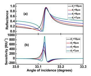
**Figure 5.**  $d_2 = 50 \ \mu\text{m}$ ,  $d_3 = 30 \ \mu\text{m}$ ,  $E_F = 0.37 \ \text{eV}$ , (**a**) Dependence of the Fano lineshape on the thickness of coupling layer  $d_1$ ; (**b**) Different values  $d_1$  corresponding to the sensitivity for the proposed sensor.
