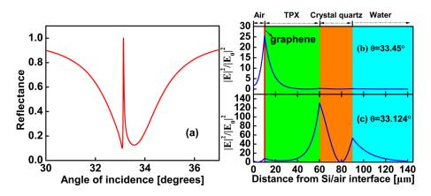
**Figure 2.** (a) ATR spectra calculated as a function of the incident angle at the  $E_F = 0.37$  eV. (b) Tangential electric field profiles (normalized by the incident light) for incident angles of 33.450°, (c) and for incident angles of 33.124°.
