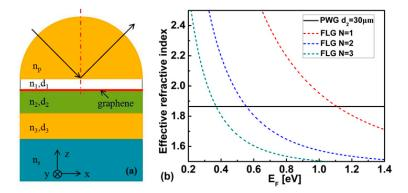
**Figure 1.** (a) Schematic diagram of the proposed biosensor based on Fano resonance; (b) Effective refractive indices of graphene SPP and PWG modes.
