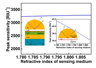
**Figure 7.** Variation of peak sensitivity with respect to refractive index of sensing medium in the vicinity of water.
