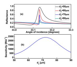
**Figure 4.**  $d_1 = 10 \ \mu\text{m}$ ,  $d_3 = 30 \ \mu\text{m}$ ,  $E_F = 0.37 \ \text{eV}$  (**a**) Dependence of the Fano lineshape on the thickness of coupling layer  $d_2$ ; (**b**) Different values  $d_2$  corresponding to the sensitivity for the proposed sensor.
