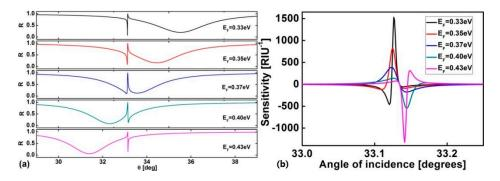
**Figure 3.** (a) Reflection spectra for different values of  $E_F$ ; (b) Different values of  $E_F$  corresponding to the sensitivity for the proposed sensor.  $E_F$  is taken to be 0.33 eV, 0.35 eV, 0.37 eV, 0.40 eV, 0.43 eV respectively.
