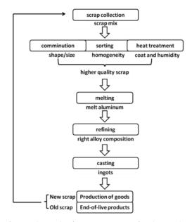
Figure 2. Flow chart of secondary Al refining operations for the production of foundry alloys.
