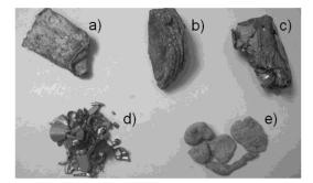
**Figure 4.** Typical Al scrap used during the charge of a rotary furnace: (**a**) wrought part; (**b**) casting; (**c**) coated packaging; (**d**) turnings and (**e**) dross.
