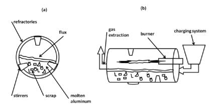
Figure 12. Draft of a rotary furnace: (a) frontal and (b) lateral view.
