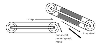
Figure 7. Overhead-belt magnetic separators.
