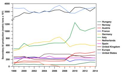
**Figure 3.** Secondary Al production from 1998 to 2014 in Europe and some European countries. The production in the USA is also reported. Data elaborated from [19].
