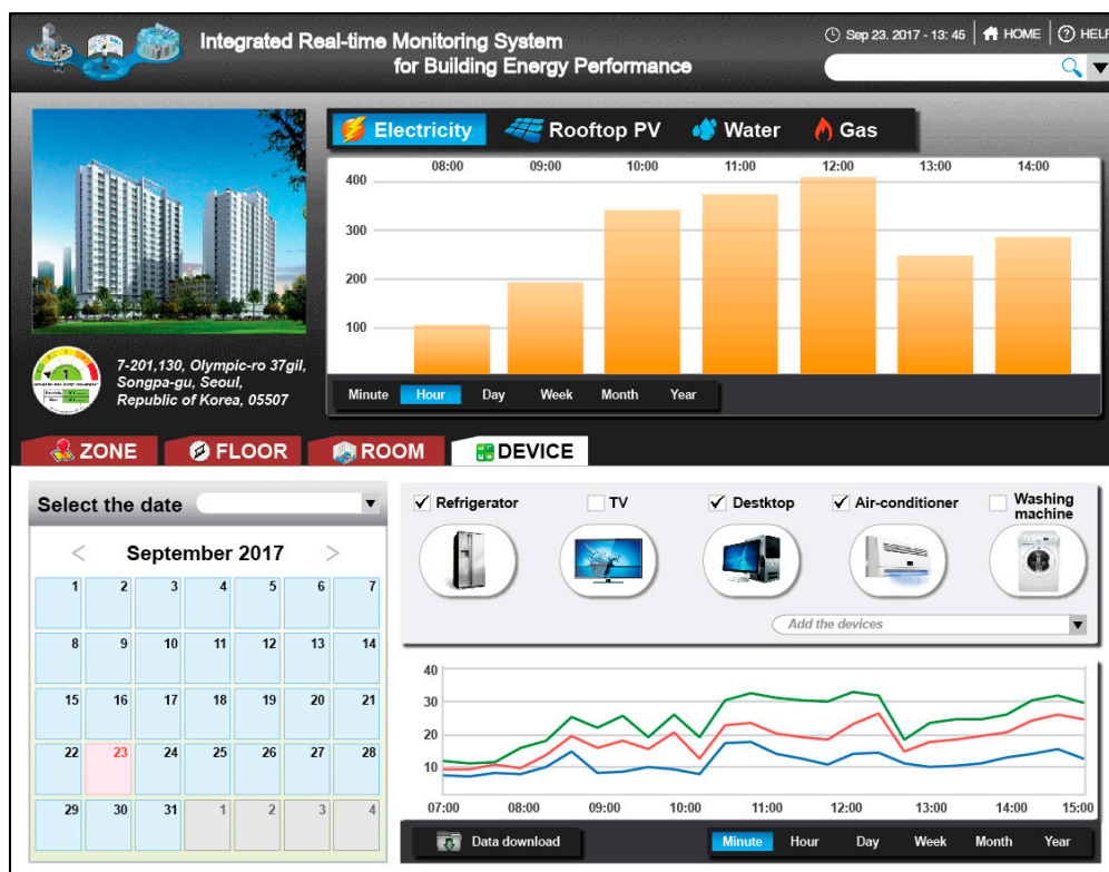
Figure 8. Integrated real-time monitoring system for the building energy performance.
