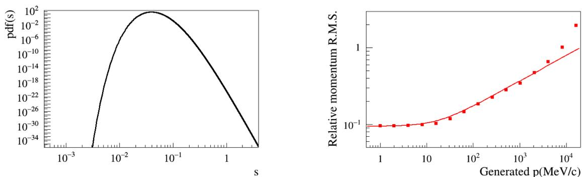
**Figure 3.** (Left) Bayesian probability density function as a function of  $s$ , the average multiple-scattering angle variance per unit track length, for a  $50 \text{ MeV}/c$  track in a silicon detector [30]. On that track, the momentum is measured to be equal to  $49.9 \text{ MeV}/c$ . (Right) The relative R.M.S of the measured momentum, as a function of the true track momentum, for a silicon detector (the curve is the parametrization of Equation (58) of [30]).
