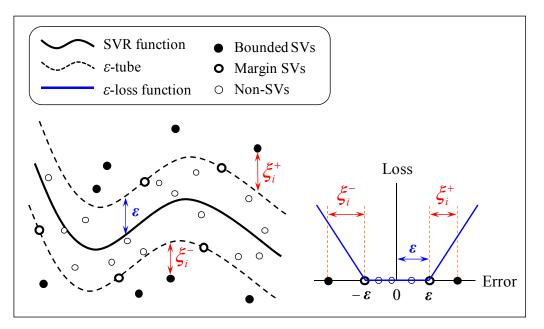
Figure 1. Illustration of SVR (modified from [11]).
