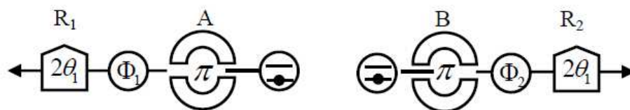
Figure 15. The schematic principle of the protocol in [54]. Both Atoms 1 and 2 are prepared in the ground state |g\rangle . The parties make them pass through a cavity, a dispersive interaction region, and a Ramsey zone, successively. The interaction times between the cavity and the atom are chosen to correspond to a \pi -pulse interaction. The phase shifts generated in the two dispersive interaction regions are controlled as \Phi_1 and \Phi_2 , respectively. The interaction times in the two Ramsey zones are chosen to correspond to the phase shifts of 2\theta_1 and 2\theta_2 , respectively.
