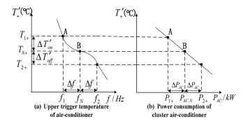
Figure 6. Frequency response characteristics of the cluster air conditioner.
