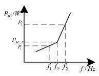
Figure 5. Frequency characteristic of cluster air conditioner.
