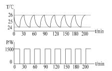
Figure 3. Power demand and temperature changes during air-conditioning operation.
