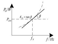
Figure 4. Frequency characteristic curve of loads.
