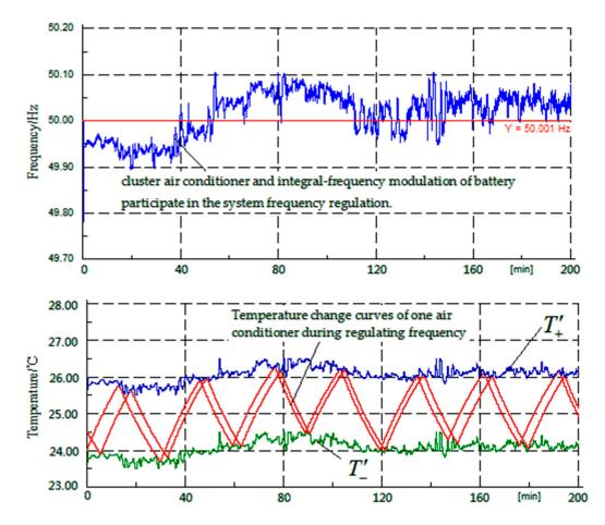
**Figure 9.** The system frequency curve and the temperature change curves of one air conditioner during the frequency regulation.
