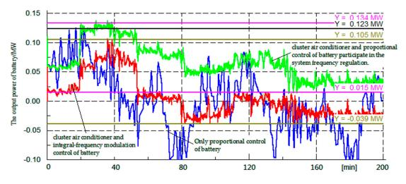
Figure 10. The power curves of battery with different frequency regulation methods.
