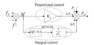
Figure 7. Integral-frequency modulation control diagram.
