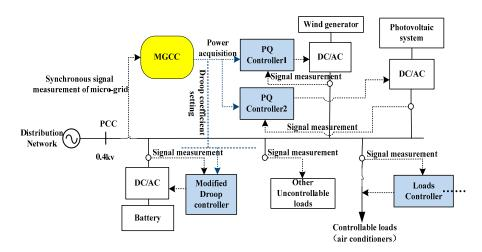
Figure 1. The hierarchical control structure of an isolated micro-grid.
