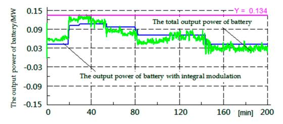
Figure 11. The output power curve of the battery.
