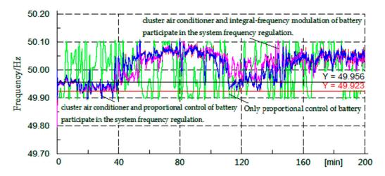
Figure 8. The system frequency curves with different frequency regulation methods of battery.
