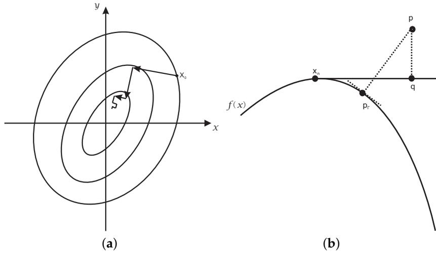
**Figure 6.** The entire graphical demonstration of Algorithm 2. (a) Step 2 of Algorithm 2; (b) Step 3 of Algorithm 2.
