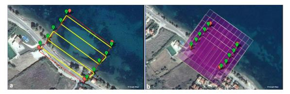
**Figure 3.** (a) Neapoli beach showing the UAV survey lines. The green pointers depict the route followed by the unmanned aerial systems (UAS) (order in-track) and the red pointers depict the four corners of the study area (mission block) (b) The overlap in-track and cross-track sidelap for image acquisition. The purple color depicts the acquired image footprint. (Map data: Google, DigitalGlobe).
