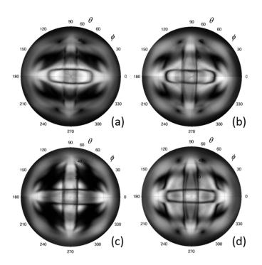
**Figure 10.** H-UPS recordings of a cross-ply C/E laminate at f = 5 MHz:  $[0^{\circ},90^{\circ},90^{\circ},0^{\circ}]$  (**a**);  $[0^{\circ},W,90^{\circ},90^{\circ},0^{\circ}]$  (**b**);  $[0^{\circ},90^{\circ},W,90^{\circ},0^{\circ}]$  (**c**) and  $[0^{\circ},W,90^{\circ},90^{\circ},W,0^{\circ}]$  (**d**). "W" stands for the position of the water-filled delamination.
