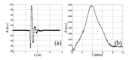
**Figure 3.** Excitation signal of a 5-MHz broadband transducer: temporal (**a**) and frequency (**b**) domain. The spectral content clearly reveals a central frequency around 4 MHz, instead of 5 MHz.
