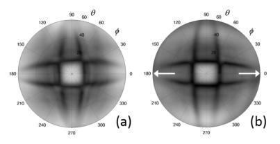
Figure 11. P-UPS recording of woven C/E laminate: before (a) and after (b) applying tension fatigue.
