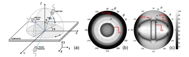
**Figure 1.** Schematic of ultrasonic polar scan (UPS) method (**a**). State-of-the-art pulsed ultrasonic polar scan (P-UPS) recordings at  $f_c = 5$  MHz: aluminum with thickness d = 0.6 mm (**b**) and  $[0^\circ]_8$  C/E laminate with thickness d = 1.1 mm (**c**). "QL", "QT-H" and "QT-V" stand for quasi-longitudinal wave and quasi-transverse wave with horizontal and vertical polarization respectively.
