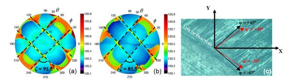
**Figure 9.** P-UPS images of  $[-45^\circ, +45^\circ]_S$  C/E laminate: before (**a**) and after (**b**) applying the shear load. Microscopic image of the fracture area when shear loading a  $[-45^\circ, +45^\circ]_S$  C/E laminate until failure (**c**).
