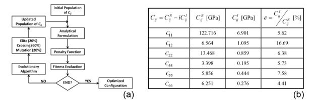
**Figure 5.** Schematic of inversion procedure to identify composite properties (**a**) and identified properties for  $[0^{\circ}]_8$  C/E laminate (**b**) [13,19]. (**a**) reproduced from [19], Copyright Society for Experimental Mechanics, 2014.
