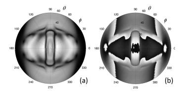
**Figure 7.** H-UPS recordings for  $[0^{\circ}]_8$  carbon/epoxy laminate at f = 5 MHz: amplitude (**a**) and phase (**b**) analysis.
