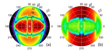
**Figure 2.** P-UPS for  $[0^{\circ}]_{8}$  C/E laminate: amplitude (**a**) and time-of-flight (TOF) (**b**) landscape [13].
