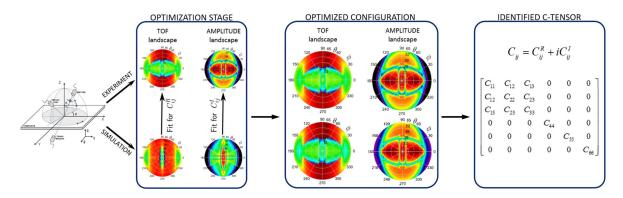
**Figure 15.** Roadmap for the identification of viscoelastic C-tensor using both TOF and amplitude P-UPS landscapes.
