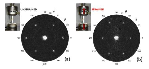
**Figure 14.** H-UBPS for DC06 steel coupon at f = 5 MHz: unstrained (a) and strained (b) state.
