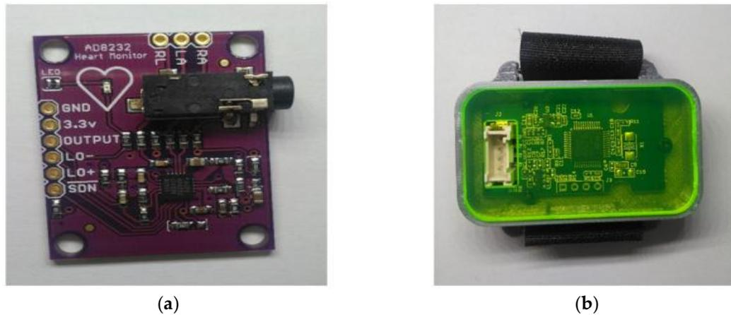
**Figure 2.** Optical biosensors: (a) electrocardiogram (ECG) heart-monitoring sensor; (b) finger-clip heart rate sensor.
