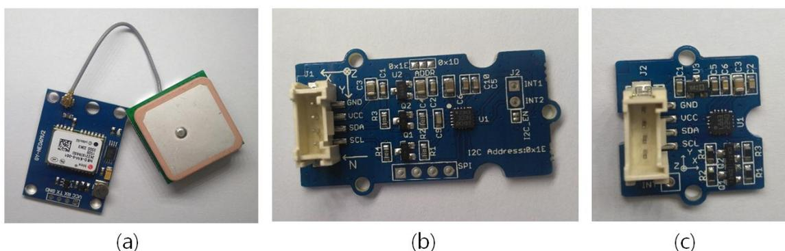
**Figure 3.** Location-tracking sensors: (a) global positioning system (GPS) module; (b) 6-axis accelerometer and compass; (c) digital compass.
