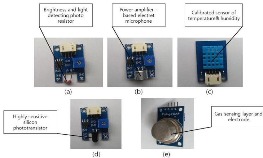
**Figure 1.** Environmental sensors and their parts: (a) light sensor; (b) sound sensor; (c) humidity sensor; (d) flame sensor; (e) fume sensor.
