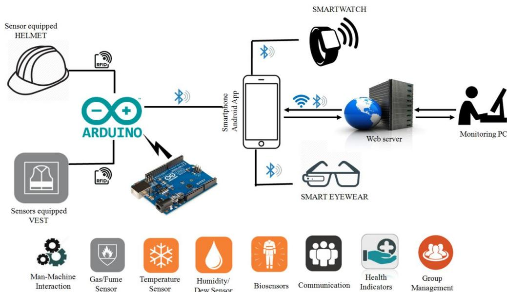
**Figure 4.** Wearable technology-integrated embedded wearable safety communication system.
