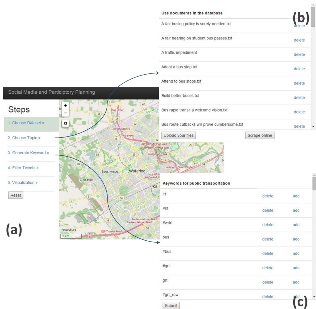
Figure 5. (a) the main interface of the TFA toolkit; (b) selecting documents for generating a customized topic lexicon; and (c) reviewing and modifying the auto-generated keyword list.
