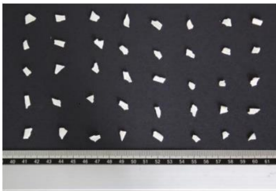
Figure 3. Picture used to compute the shape factor of MATER-BI 2-WF particles belonging to size class II.
