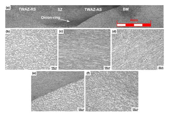
**Figure 4.** Optical microscopy of cross section of the joint (**a**); related microstructure (**b**) base metal (BM); (**c**) stir zone (SZ); (**d**) stir zone—advancing side (SZ-AS); (**e**) thermo-mechanically affected zone—advancing side (TMAZ-AS); (**f**) thermo-mechanically affected zone—retreating side (TMAZ-RS).
