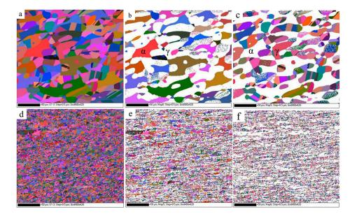
**Figure 6.** EBSD maps of the BM and the SZ: (**a**) map for the BM; (**b**) ferrite of the BM; (**c**) austenite of the BM; (**d**) map for the SZ; (**e**) ferrite of the SZ; (**f**) austenite of the SZ.
