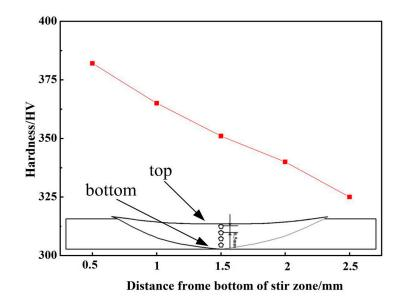
Figure 9. Hardness profile along the weld thickness.
