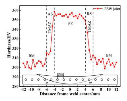
Figure 8. Hardness profile across the joint.
