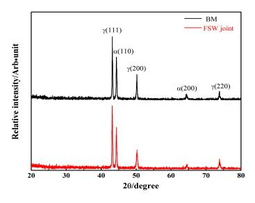
Figure 7. XRD pattern of base metal and SZ.
