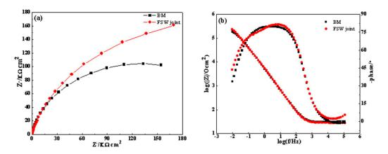
Figure 14. Nyquist (a); and Bode (b) plots for the BM and the SZ in a 3.5 wt. % NaCl solution.
