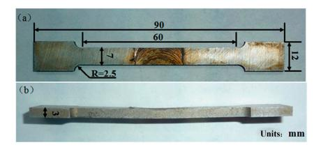
Figure 3. (a) The front; (b) sectional views of the transverse tensile specimen.
