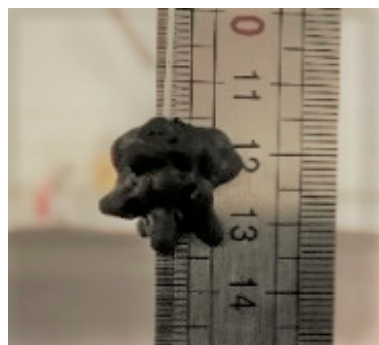
Figure 5. The tumor phantom: microlobulated shape, average radius of 14 mm, dielectric properties matching the measured dielectric properties of excised malignant tissue.
