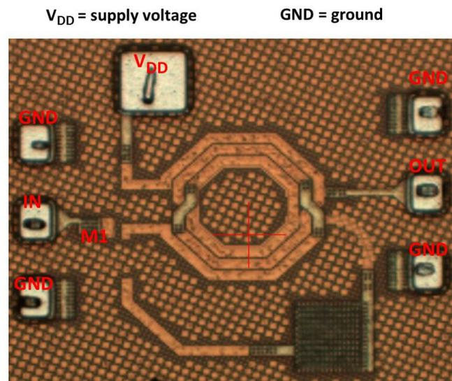
Figure 7. Microphotograph of the implemented power amplifier
