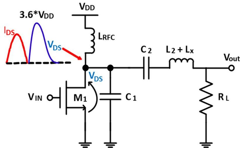
**Figure 1.** Conventional Class-E power amplifier (PA) using NMOS transistor with radio frequency RF-choke and series LC network.
