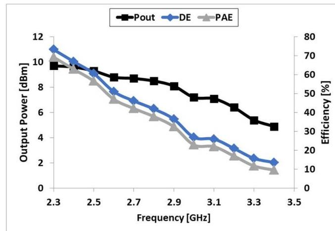
**Figure 10.** Transformer-based class-E PA: Measured output power, drain efficiency and power-added efficiency versus operating frequency.
