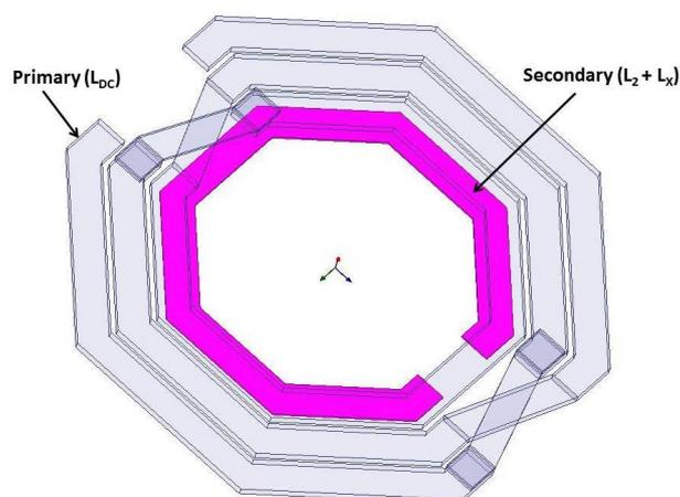
Figure 5. Schematic of on-chip transformer 3-D view
