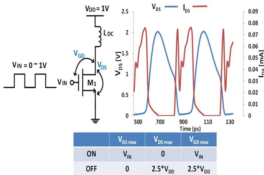
Figure 4. Maximum voltage stresses on transistor M1 in both on and off states.
