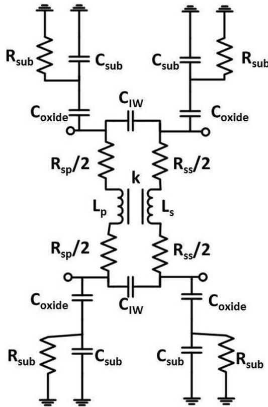
Figure 3. Basic model of transformer.
