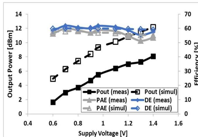
**Figure 9.** Uncoupled class-E PA: Output power, drain efficiency and power-added efficiency versus the dc supply voltage (measurement: solid black, blue and grey; simulation: dashed white, blue and grey). Drain efficiency (DE) and power-added efficiency (PAE)
