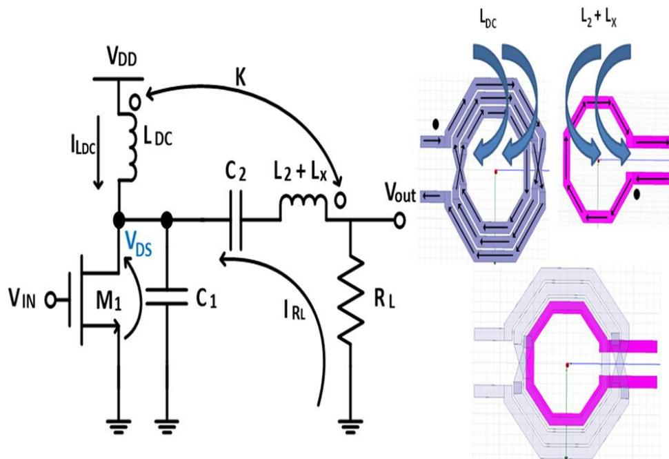
Figure 2. Transformer-Based Class-E PA: magnetic coupling and determining correct dot placement.
