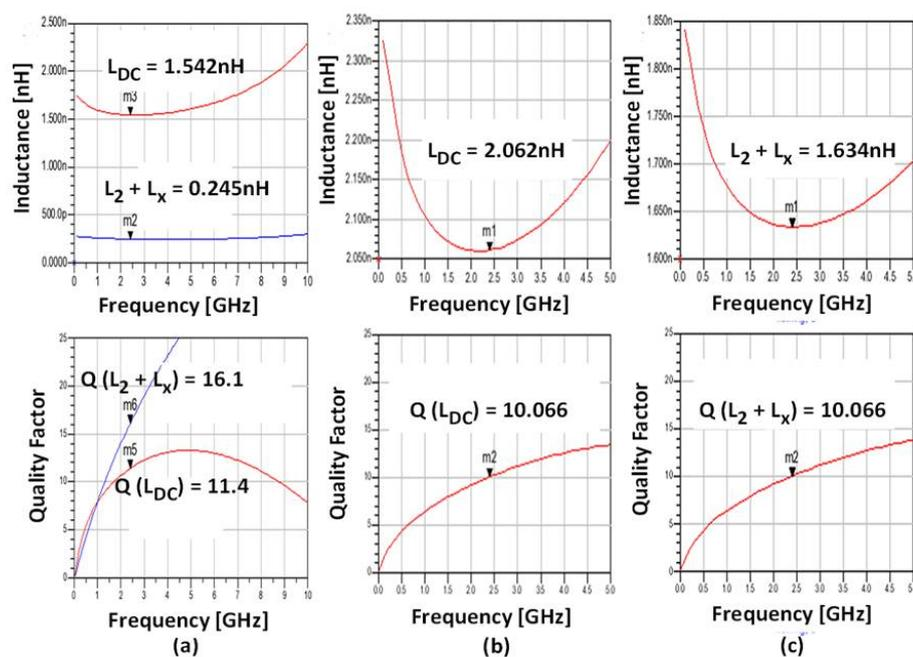
Figure 6. The quality factor plotted versus frequency for the inductors: (a) Coupling-inductors; (b) DC-feed inductor; (c) Output series inductor.
