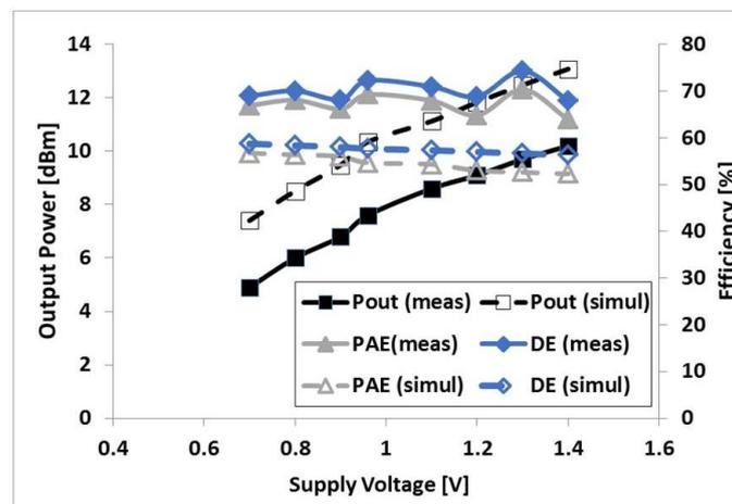
Figure 8. Transformer-based class-E PA: Output power, drain efficiency and power-added efficiency versus the DC supply voltage (measurement: solid black, blue and grey; simulation: dashed white, blue and grey).
