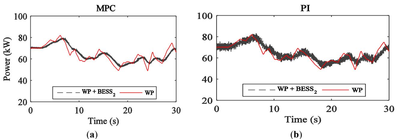
**Figure 6.** Smoothed wind power: (a) MPC technique; (b) PI technique.
