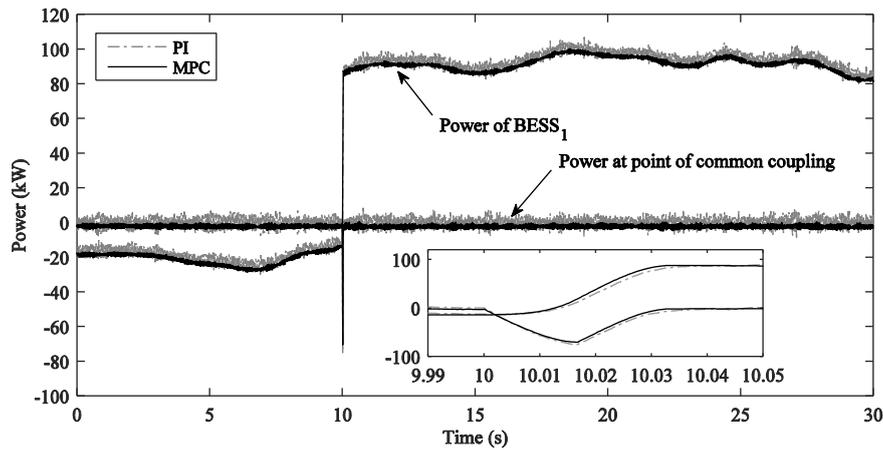
Figure 7. Real power at point of common coupling and real power of BESS<sub>1</sub>.
