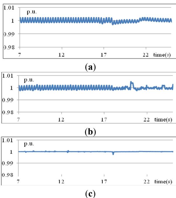
**Figure 10.** Voltages at bus 3 obtained using three methods: (a) traditional PID; (b) T1 fuzzy rules; and (c) IT2 fuzzy rules (Scenario 2).
