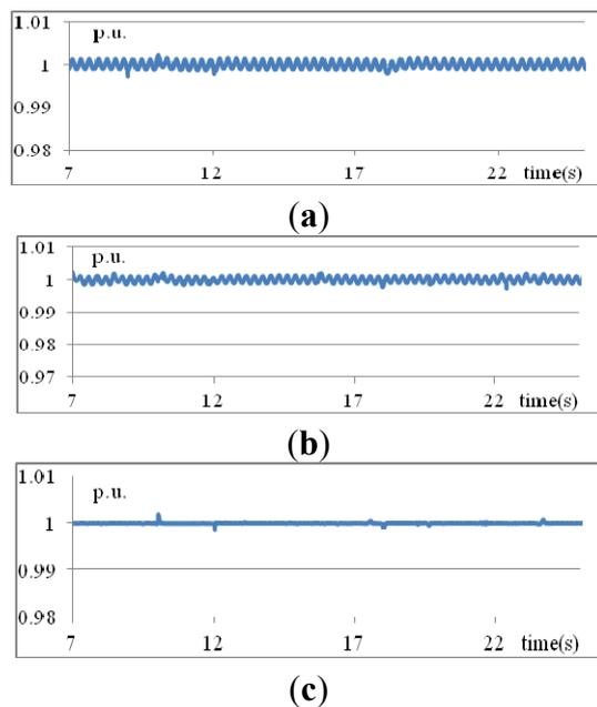
**Figure 13.** Voltages at bus 3 using obtained three methods: (a) traditional PID; (b) T1 fuzzy rules; (c) IT2 fuzzy rules (Scenario 3).
