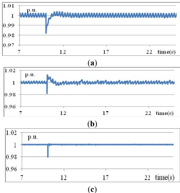
**Figure 7.** Voltages at bus 3 obtained using three methods: (a) traditional PID; (b) T1 fuzzy rules; (c) IT2 fuzzy rules (Scenario 1).
