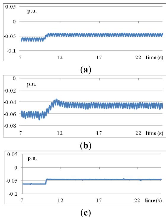
**Figure 16.** MVARs from STATCOM obtained using three methods: (a) traditional PID; (b) T1 fuzzy rules; and (c) IT2 fuzzy rules (Scenario 4).
