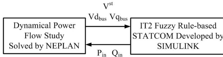
**Figure 5.** Co-simulation conducted by integrating NEPLAN with Simulink.
