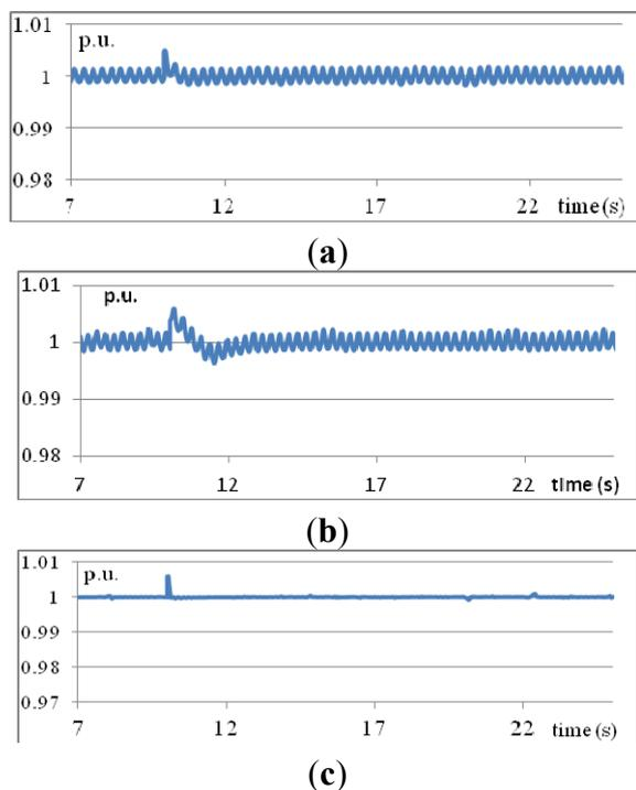
**Figure 15.** Voltages at bus 3 obtained using three methods: (a) traditional PID; (b) T1 fuzzy rules; (c) IT2 fuzzy rules (Scenario 4).
