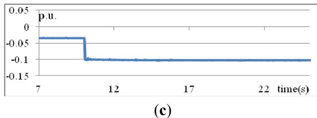
**Figure 8.** MVARs from STATCOM obtained using three methods: (a) traditional PID; (b) T1 fuzzy rules; (c) IT2 fuzzy rules (Scenario 1).
