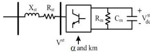
Figure 3. Model of static synchronous compensator (STATCOM).
