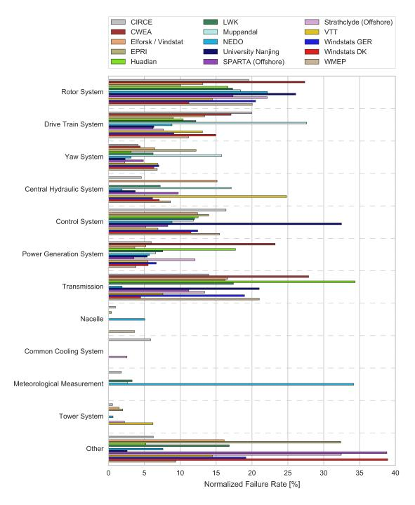
Figure 7. Normalized failure rates per system as published by different initiatives.
