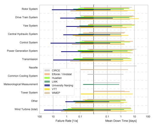
Figure 6. Overview on failure rate and mean down time per WT as published by different initiatives.
