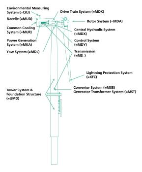
**Figure 5.** System structure of a WT according to the Reference Designation System for Power Plants (RDS-PP<sup>®</sup>) published by VGB PowerTech [66]. The figure does not provide a complete overview on the system structure but highlights the most important systems considered in this paper.
