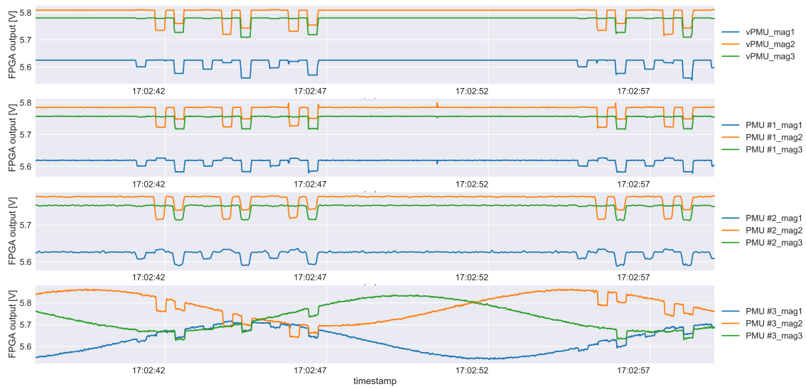
Figure 11. Comparison of measurements of three real PMUs and vPMU under a 50 \Omega impedance fault.
