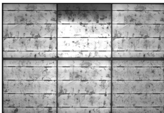
Figure 6. EL image at 100% I_{SC} of a test module with a defective cell interconnection in the original state.
