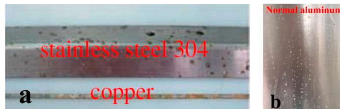
Figure 1. Corrosion phenomenon of liquid desiccant on metals: (a) stainless steel (b) aluminum.
