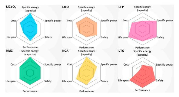
**Figure 4.** Comparisons of different types of Li-ion batteries used in EVs from the following perspectives: specific energy (capacity), specific power, safety, performance, life span, and cost (the outer hexagon is most desirable). Lithium Nickel Manganese Cobalt Oxide (NMC), Lithium Iron Phosphate (LiFePO<sub>4</sub>) and Lithium Manganese Oxide stand out as being superior among these six candidates [26].
