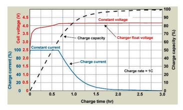
Figure 6. Example Constant Current, Constant Voltage (CC-CV) battery charging approaches [106].
