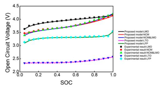
**Figure 5.** The estimated and experimental OCV curves for different Li-ion batteries: LiMn $_2$ O $_4$  (LMO), Li(Ni $_x$ Mn $_y$ Co $_{1-x-y}$ )O $_2$  (NCM or LNMCO), NCM&LMO, LiTi $_5$ O $_{12}$  (LTO), LiFePO $_4$  (LFP) [103].
