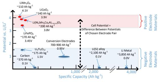
**Figure 3.** A summary of some present and future electrode chemistry options for Li-ion batteries. The proposed capacity of the Li(Si) is 50% of the theoretical capacity of the material, similar to the case found for some of the positive electrode materials.
