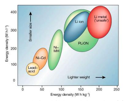
Figure 1. Ragone plot of several of the battery technologies used in EVs [12].
