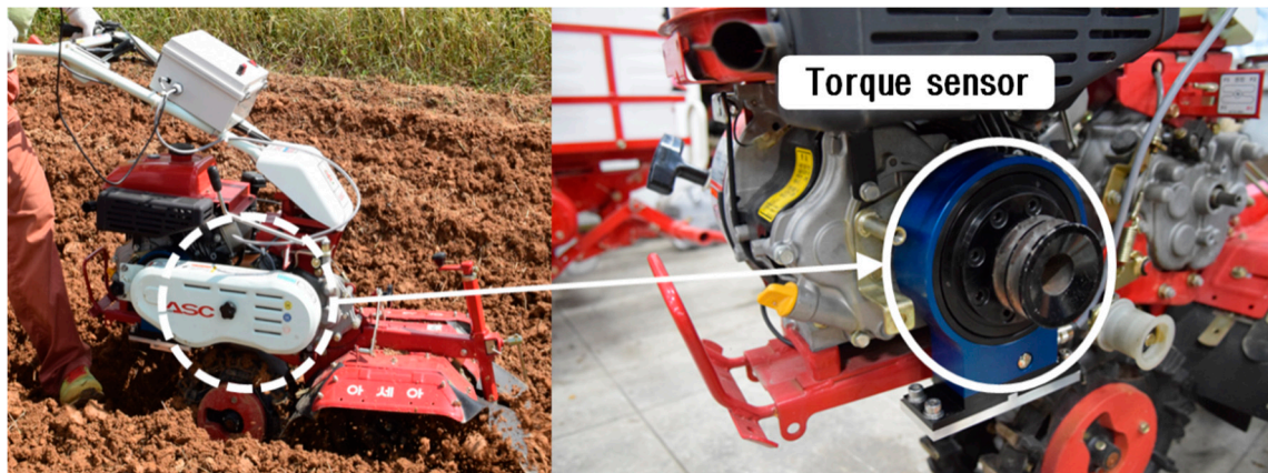
Figure 2. Torque measurement system for the cultivator.
