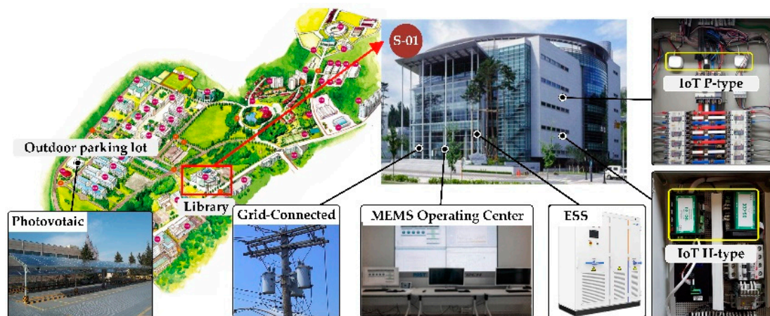
Figure 1. Architecture of the implemented IoT-based campus MG.
