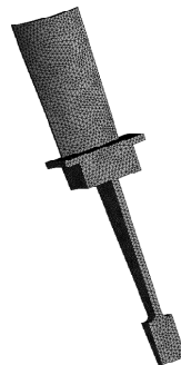
Figure 5. Finite element (FE) model of turbine blisk.
