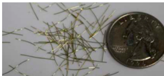
Figure 5. Steel fibers with slightly deformed mid-section [7].
