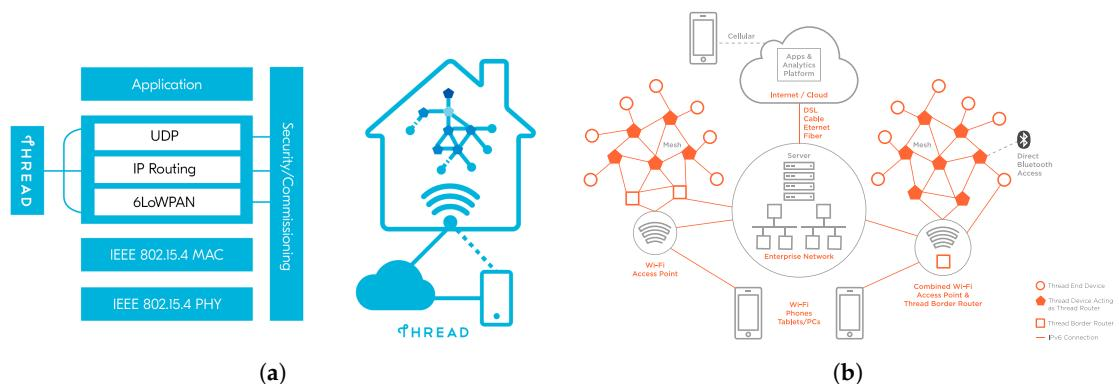
**Figure 5.** Protocol stack and network architecture representation of an infrastructure handled with Thread protocol. (a) Thread networking protocol stack [69]; (b) Thread network architecture example [70].
