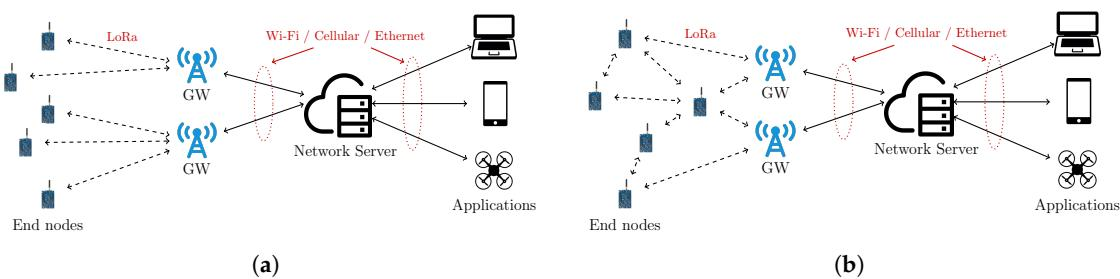
**Figure 7.** LoRaWAN network topology. (a) Star of star topology in LoRaWAN network; (b) Mesh topology in LoRaWAN network.
