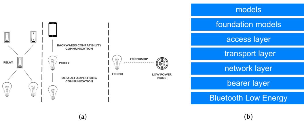
**Figure 4.** Examples of optional features within the Bluetooth Mesh standard and protocol stack. (a) Examples of optional features within the Bluetooth Mesh standard; (b) BLE protocol stack.
