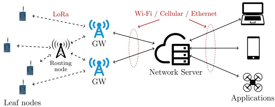
**Figure 11.** LoRa-based network with intermediate relay.
