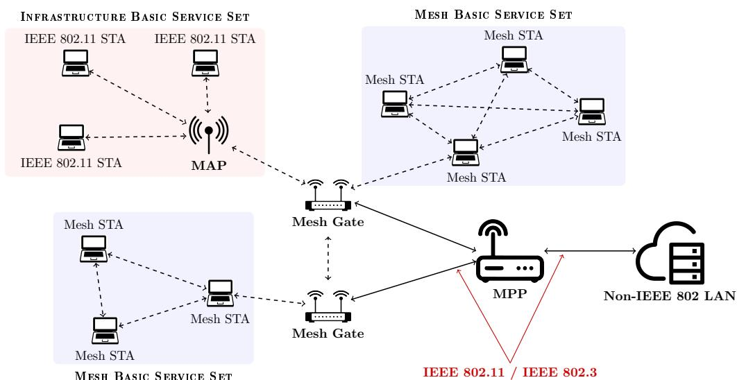
**Figure 1.** Architecture of MBSS containing mesh STAs, APs and portals as designed in IEEE 802.11s standard [8].
