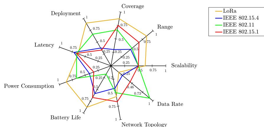
**Figure 17.** Comparative performance analysis, with 9 relevant metrics, of 4 wireless mesh technologies.
