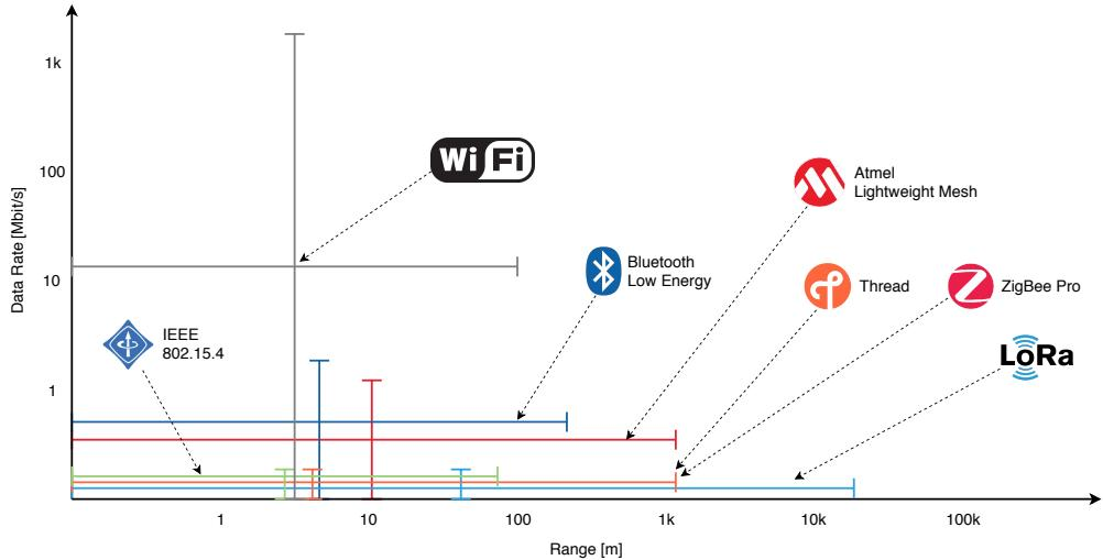
**Figure 16.** Comparison among the analyzed communication protocols, based on data rate and transmission range. Minimum and maximum values (with average) are indicated for each performance metric.
