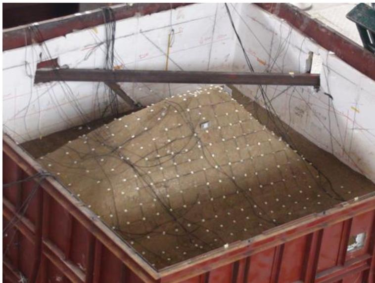
**Figure 4.** Shaking table test model of an isolated slope.
