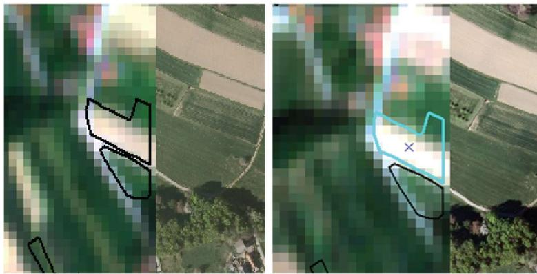
**Figure 10.** S-2 images (left: 2016 growing season, right: 2017 growing season) provided additional information to confirm problematic dates of changes for a particular object (object no. 2). Digital orthophoto in the background with 1 m spatial resolution, but single date land use state information (April 2016).
