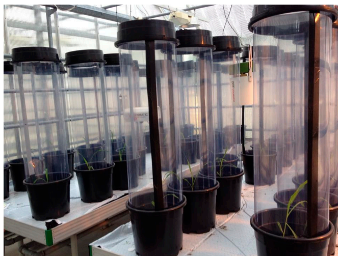
Figure 1. Experimental cages made of plastic Mylar film. Cage tops were covered with fine nylon mesh and secured with plastic rings to prevent insect escape.
